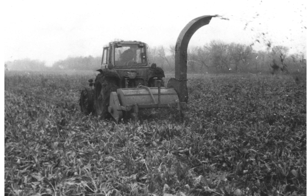
Fig. 2. Operation of haulm removing machine with improved loading mechanism under field conditions
